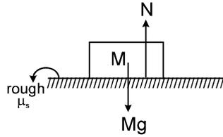
**Sol.** In horizontal direction as acceleration is zero. Therefore  $\Sigma F = 0 \therefore f = 0$
