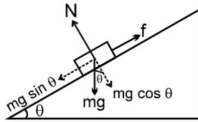
As the block is at rest, these forces should add up to zero. Also, since  $\theta$  is the maximum angle to prevent slipping, this is a case of limiting equilibrium therefore  $f = \mu_s N$
