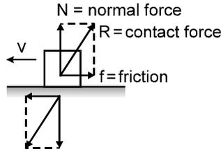
The direction of the contact force acting on a particular body is not necessarily perpendicular to the contact surface. We can resolve this contact force into two components, one perpendicular to the contact surface and the other parallel to it (figure). The perpendicular component is called the normal contact force or normal force (generally written as N) and the parallel component is called friction (generally written as f).
