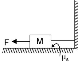
**Sol.** As the external force  $F$  is gradually increased from zero it is compensated by the friction and the string bears no tension. When limiting friction is achieved by increasing force  $F$  to a value till  $\mu_s mg$ , the further increase in  $F$  is transferred to the string.
