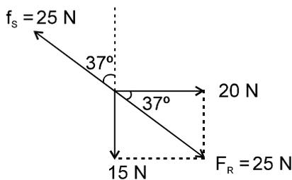
As the object does not move this is not a case of limiting friction. The direction of static friction is opposite to the direction of the resultant force  $F_R$  as shown in figure by  $f_s$ . Its magnitude is equal to 25 N.
