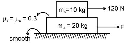
**Ans.** In the above situation we see that the maximum possible value of friction between the blocks is  $\mu_s m_A g = 0.3 \times 10 \times 10 = 30 \text{ N}$ .
